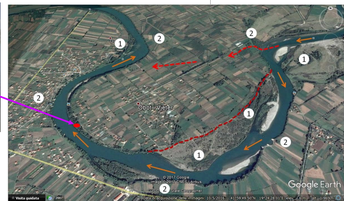
-----> Normal river stream -----> Flood streams -----> Ancient right bank of the river ① Debris Deposit ② Eroded river bank
